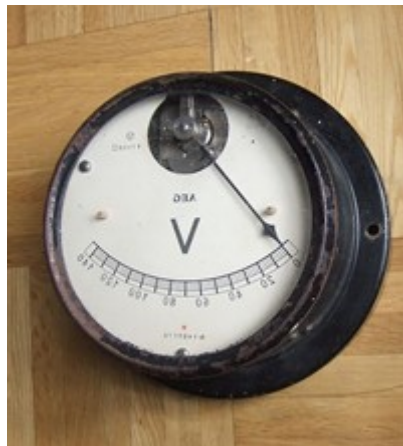
Figure 1: A voltmeter (left) and the symbol for a voltmeter in a circuit diagram (right)
