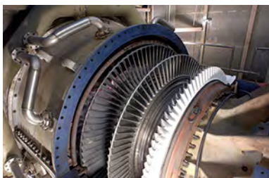
Figure 20.29 Steam turbine generator. The steam produced by burning coal impacts the turbine blades, turning the shaft which is connected to the generator. (credit: Nabonaco, Wikimedia Commons)
