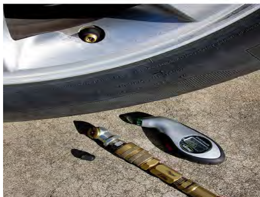
Two more complicated types of tyre pressure gauges for measuring the air pressure inside car tyres. The right one is a digital gauge.
